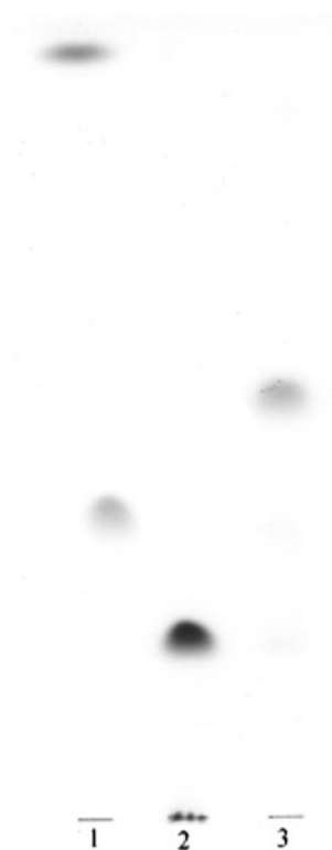
Fig. 1 TLC of starting materials, an intermediate (oleoyl-2-methylpropanol amide), and the final product (oleic acid DMOX). Lane 1 standard FFA and ME of oleic acid, Lane 2 oleoyl-2-methylpropanol amide, Lane 3 DMOX derivative of oleic acid. Solvent system: chloroform/acetone (8:2, by v/v). Detection: charring at 110 °C after spraying with 5% H 2 SO 4 in methanol
